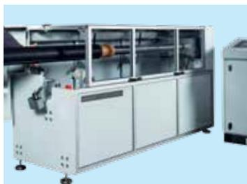
Automatic air flow on cylinder facilitates easy loading of sleeves and adapters.
