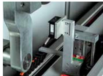
Scanner laser sensor measures high or low spots and relief on sleeves with variable speed to verify sleeve quality.
