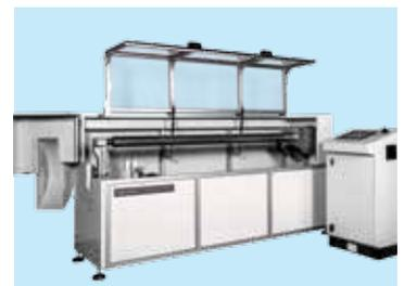
Top lid provides easy visual inspection and maximum safety during scanning operations.
